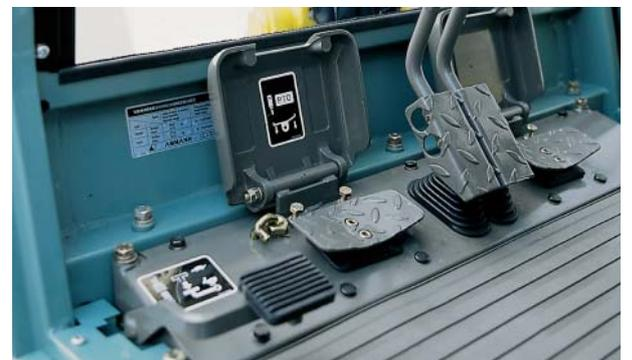
Separated pedals for 3rd circuit and boom swing fitted with robust protections on pedal guards acting as footrests.
